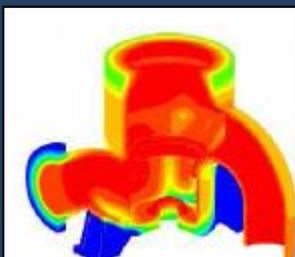
a/ Valve casing – Temperature distribution
